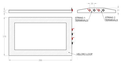
Arrays consist of two identical solar cell strings, each wired to a positive red (Jaycar PS-0406) and negative black (Jaycar PS-0408) 4mm banana socket terminal, and teams are free to connect these in either series or parallel as desired. A typical electrical output of the two strings configured in series is given below:
